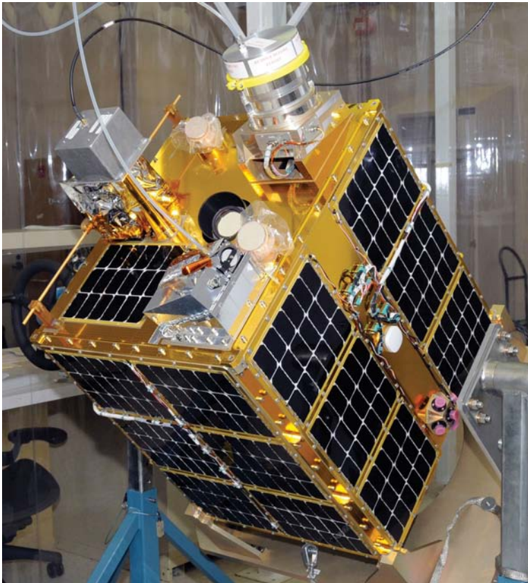
Figure 33. Small satellites composed from standardized modular elements can provide rapid on-orbit capabilities with “good enough” functionality. Fractionated or distributed space systems composed from such small satellites can significantly increase their functionality and survivability. (Courtesy NASA.)
