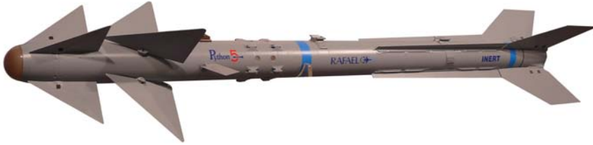
Figure 9. Dual-mode EO-IR focal-plane array seeker technology, as on the Python-5 AAM, can give wide field-of-view imaging infrared capability and full-sphere beyond-visual-range engagement. (Reprinted from Wikipedia , s.v. "Python [missile]," accessed 20 June 2011, http://en.wikipedia.org/wiki/Python_(missile) .)
